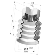
Bellows Suction Cup 4.5 folds Series 92, Ø 20 mm Product reference: 92 20-- FM5GIC
