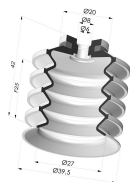
Bellows Suction Cup 4.5 folds Series 92, Ø 40 mm
